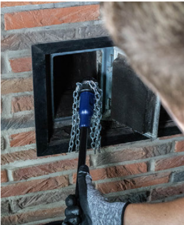
The universal rotary head can be equipped with chains. So even persistent soot is no longer a problem for you.
